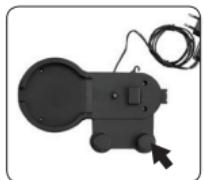
To disconnect your appliance from the charging stand, press the button on the stand and pull the appliance towards you.
