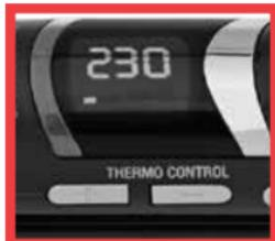
To deactivate the locking temperature function, press "+" and "-"buttons simultaneously again. The "lock" symbol will disappear on LCD display.
